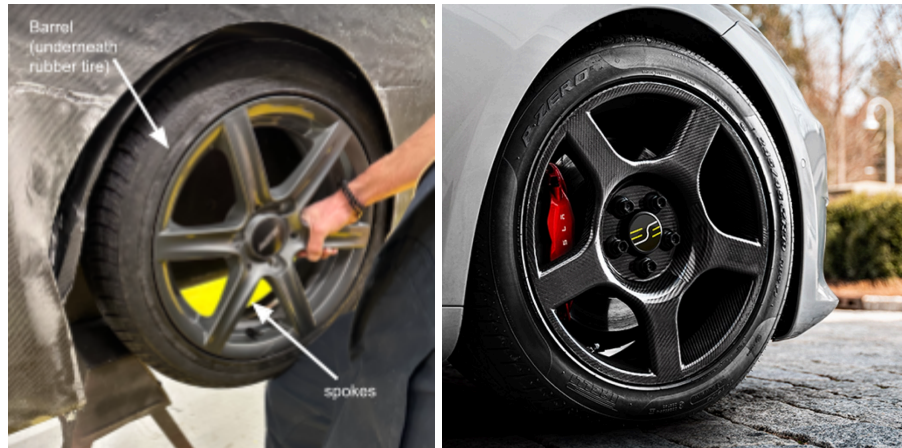
Figure 4-5: Current (Aluminum) tires used for the 2024 SEM (left) vs example of a market carbon fiber rim, sold by ESE Carbon (right)
